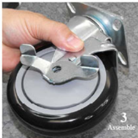
(3). Insert wheel into yoke & Brake Lever over the Brake Arm; aligning the axle holes of each part.
