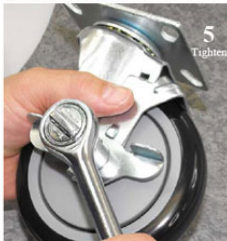
(5). Using a wrench, tighten nut onto the axle until all parts are firmly held together. Make sure not to over tighten. Wheel should still be able to spin freely and brake arm should be able to slide from the on to the off positions.
