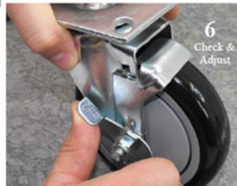
(6). Check to make sure Brake Lever is not loose (parts should not be able to move or jiggle without force). Or too tight; so as to prevent brake from working. Make slight adjustments in the tightness of the nut, until brake works satisfactory.
