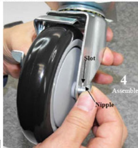
(4). While holding all parts together insert axle, with the axle head opposite the brake parts (threads facing brake side) Make sure the nipple on the underside of the axle head fits into the slot on the axle hole of the caster yoke (this will keep the axle in place and prevent it from turning when tightening the nut). Thread nut onto the axle and finger tighten.
